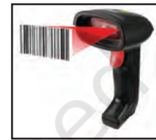
Figure 1.12: Capturing data using barcode reader
